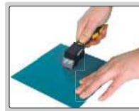
step 1: make grid cutting on surface
