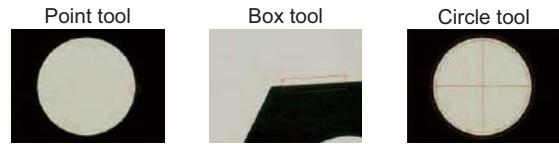
Input CAD drawing and set reference, move the stage to make the target box in the center of crosshair, then the software will do automatic measurement
