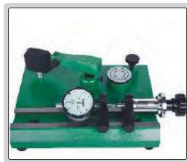
inspect accuracy of dial indicators (range 0-25mm)
